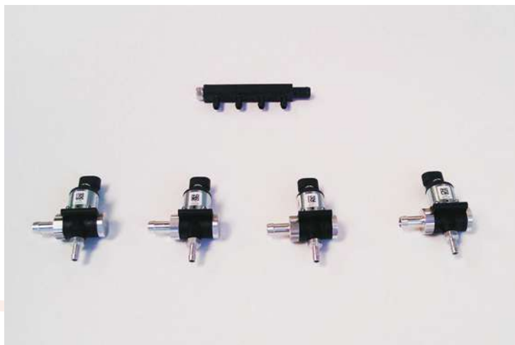
IG3 Horizon injectors (single injector for each cylinder)
